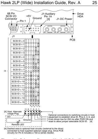
Figure 3b. Drive configurator Hawk 2LP family W/WD models
