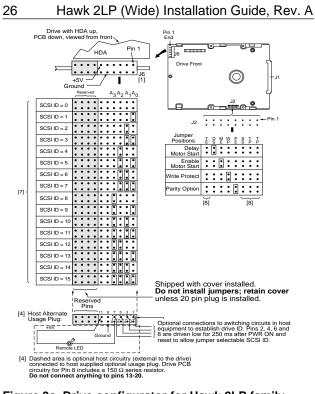
Figure 3c. Drive configurator for Hawk 2LP family WC/DC models
