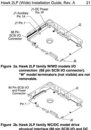
physical interface (80 pin SCSI I/O and DC power connector). Terminators are not provided.
