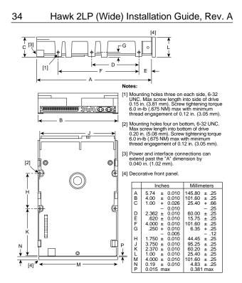
Figure 4. Hawk 2LP family W/WD model drive mounting dimensions (68 pin SCSI I/O connector)
