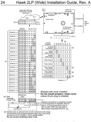
Figure 3a. Drive configurator Hawk 2LP family W/WD model
